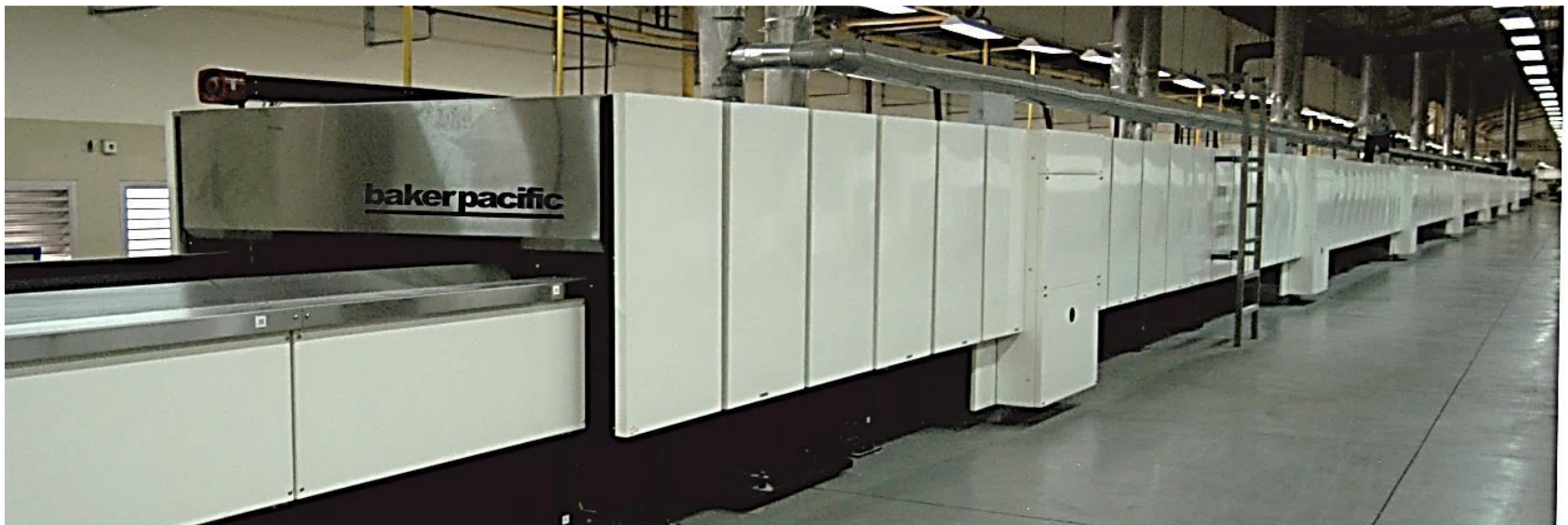
1.2m x 100m Indirect Radiant oven built in India
